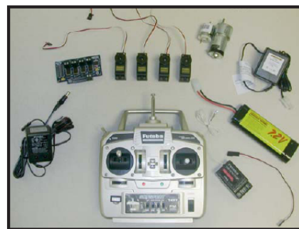
The Advanced DSP Education Kits support radio control of the DSP and capability for the DSP to control motors and servos
