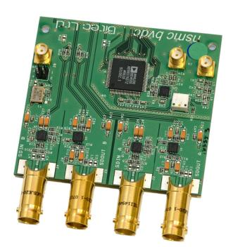
The BVDC is designed for professional video equipment developers. The dual ASI/SD-SDI interfaces allows FPGA designs access to industry standard video transport signals. Based on the latest adaptive cable equalizers and drivers, the ASI/SDI interfaces produces excellent noise immunity up to cable lengths of 350m. A VCXO allows precise synchronisation to incoming ASI signals.
