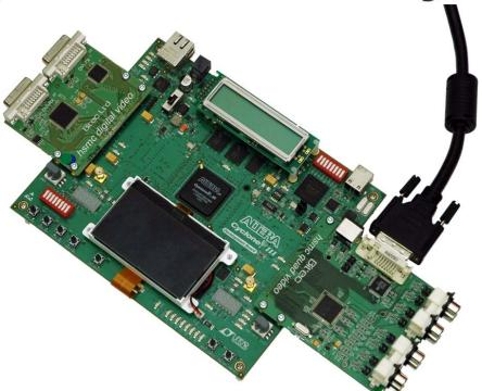
The Cyclone III is an ideal video processing platform given the large number of multipliers, low power and M9K memory blocks. The Bitec Video Development Kit provides a cost effective, integrated solution for developers wishing to utilise the Cyclone III device for video application development. Based on the Altera Cyclone Development Kit, the Video Development Kit enables designs to interface to a wide variety of video devices via two High-Speed Mezzanine Connector (HSMC) daughter cards.
