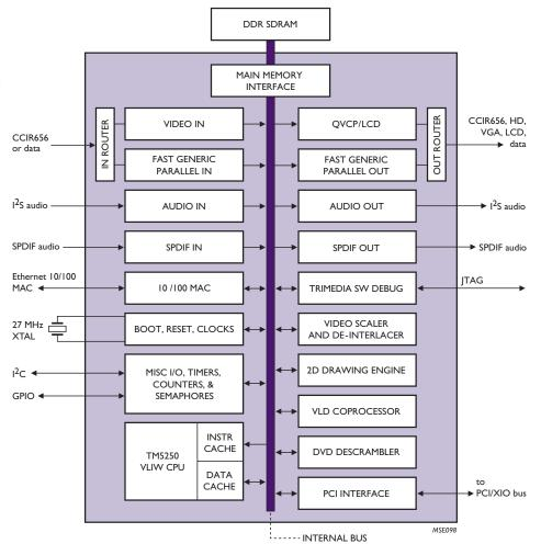
The CPU's five issue slots enable up to five simultaneous RISC-like operations to be scheduled into only one VLIW instruction. These operations can simultaneously target any five of the CPU's 30 pipelined functional units within one clock cycle.
