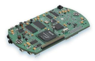
direct LCD output and supports video resolutions up to WXGA TFT LCD (1280  $\times$  768 60 Hz) or SD/HD video (up to 1920  $\times$  1080 60i). For generating high-quality video on internal or external displays, the PNX1500 handles high-definition video scaling, linear and non-linear aspect ratio conversion, anti-flicker filtering, brightness control, and a long list of video quality enhancements.
