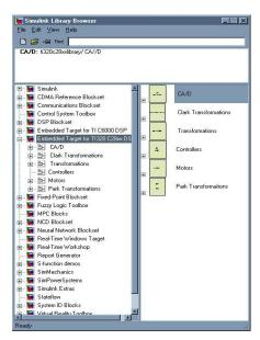
TI320C28xxtarget : target file used to generate C code for real time implementation
