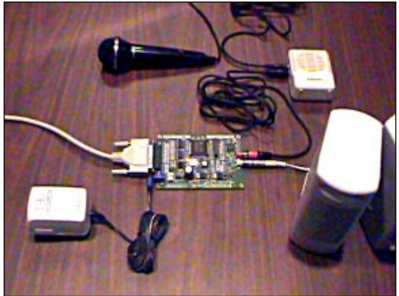
Real-time DSP hardware setup with speakers, microphone, and power supply
