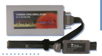
The new Blackhawk USB560 is the second generation of the widely used XDS560-class emulator first introduced by Blackhawk and the only USB JTAG Emulator that supports all of the advanced capabilities of Texas Instruments latest DSPs. These capabilities include high-speed Real-Time Data Exchange (RTDX)™, for lightning speed downloads and Advanced Event Triggering to quickly find and fix real-time software problems.
