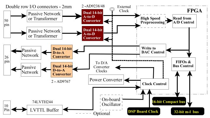
The FPGA provides for a number of interface functions in the peripheral card.
