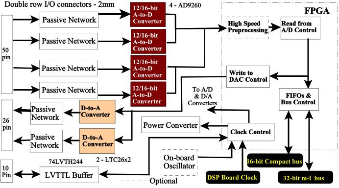
The FPGA provides for a number of interface functions in the peripheral card.
