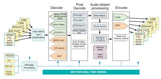
The Performance Audio Framework (PA/F), pictured at right, creates a modular software development environment. Drivers, codecs, and processing can be inserted into the chain without disrupting the environment.
