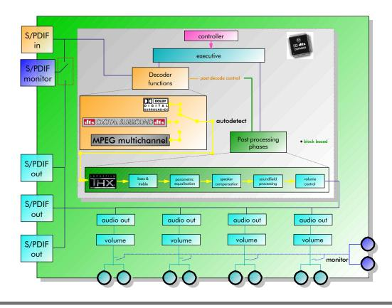
The <u>Digital Audio Engine</u> itself is a compact, 'off the shelf' module which includes all the digital processing needed fo rmultichannel audio decdoing, as well as the high quality analog audio reconstruction.
