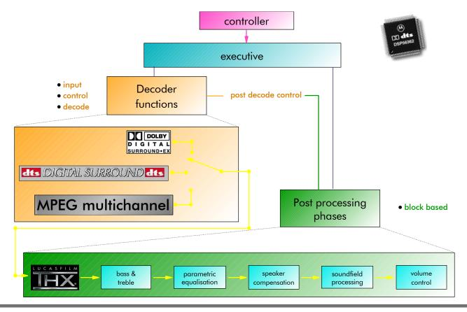
In addition to the hardware, the <u>DSP56362</u> has a defined software architecture which aims to make it <u>easier for</u> programmers to control standard functions and to add new post processing phases.
