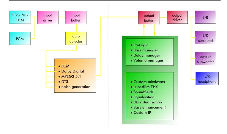
The incoming multichannel audio bitstream can be in various formats. DVDs provide <u>Dolby Digital</u>, <u>DTS</u> and <u>MPEG2</u> sound tracks: multichannel CDs may also use <u>DTS</u> or <u>HDCD</u>, and there may also be conventional PCM audio.
