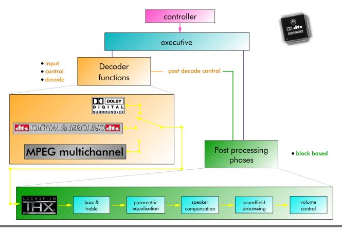
The executive invokes each active PPP in turn. The PPPs process the data in place (that is, their output overwrites the input data buffer). After all PPPs have been executed, the channels are paired (left/right, centre/sub woofer, left and right surround) and transmitted by the Enhanced Serial Audio Interface to external DACs.
