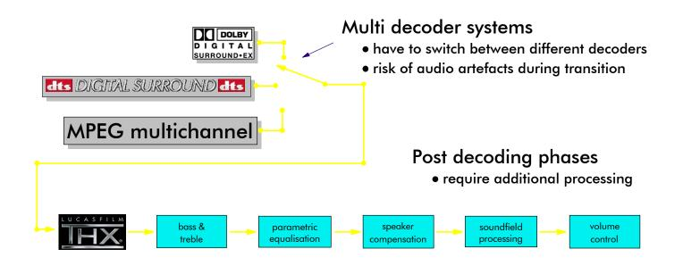
Multichannel audio standards and products are evolving quickly: consumers and manufacturers alike want to products that support all the primary standards while at the same time allowing for new or custom affects. Multi decoder systems have to switch between the different decoders: when they do so there is a risk of audio switching artefacts so the switching has to be handled smoothly - this requires some processing power.
