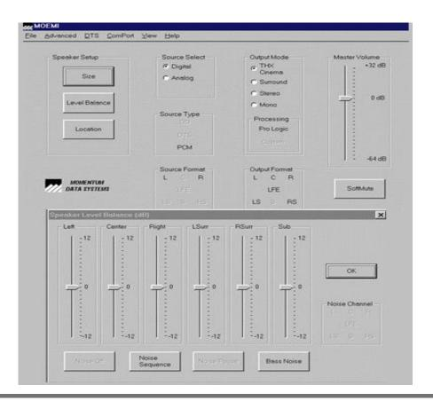
The Momentum OEM Interface (MOEMI) provides a **ready made software interface** to control the <u>Digital Audio Engine</u> (via a <u>Digital audio Development Environment</u> (DDE) from a PC using the RS232 serial port.
