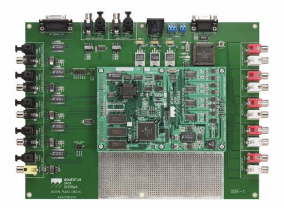
The Digital audio Development Environment (DDE) provides a **ready made base** so that the <u>Digital Audio Engine</u> modules can be used immediately for **development and testing**.
