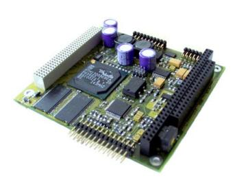
The TriMeleon DT1304 Board is a compact, high performance board for video, audio and telecommunications applications. It integrates on a small area (standard PC/104 format) the Philips TriMedia® TM1300 Multimedia Processor, 32 Mbytes SDRAM, analog audio and video I/O interfaces including all necessary A/D and D/A converters.
