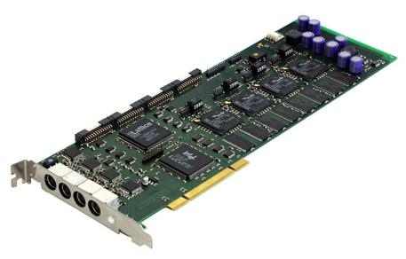
The TriMeleon DT1341 Board is a full size PCI high performance board for video applications. It integrates four Philips TriMedia® TM1300 Multimedia Processors, with 16 Mbytes of SDRAM each, analog video I/O interfaces including all necessary A/D and D/A converters.
